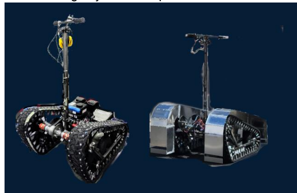
Figure 1: ICE-powered on left, electric with shields on right
